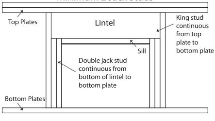
These spans are generated using Manitoba Building Code span Tables and cwc 2004 span tables forming part of MBC 9.23, with an assumed snow load of 2.0 kpa and 4/12 roof slope. The lintel tables below indicate size of openings and acceptable lintel spans. For additional sizes and spans, please refer to the Manitoba Building Code span tables.
